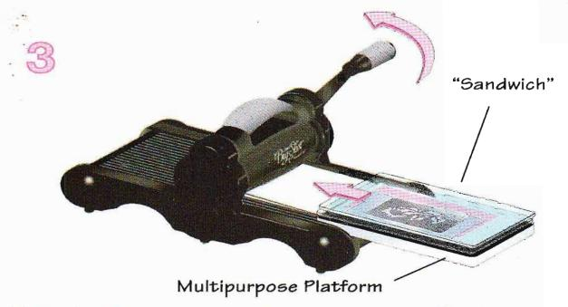
3. Place the sandwich on top of the Multipurpose Platform and slide both together into the opening of the Big Shot. Note the rotation of the handle and continue to rotate it in the same direction until the sandwich and Multipurpose Platform have passed through the opening and rollers. Remove the Platform from Big Shot, and your embossed design is ready to use!
