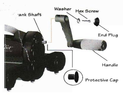
Before attaching handle, remove protective cap on crank shaft and discard. Then attach handle by sliding washer over hex screw and inserting through handle and into crank shaft. Tighten hex screw with hex wrench provided with handle kit. Press end plug over hex screw until firmly sealed.
