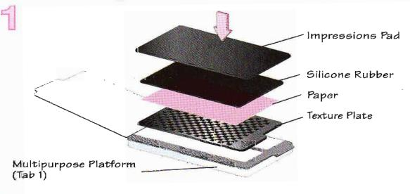
1. Flace a Texture Plate directly on Tab 1 of the Multipurpose Platform with the desired design facing up. Place paper or desired material on top of Texture Plate. Place Silicone Rubber on top of paper. Place Impressions Pad on top of Silicone Rubber to create a "sandwich."
