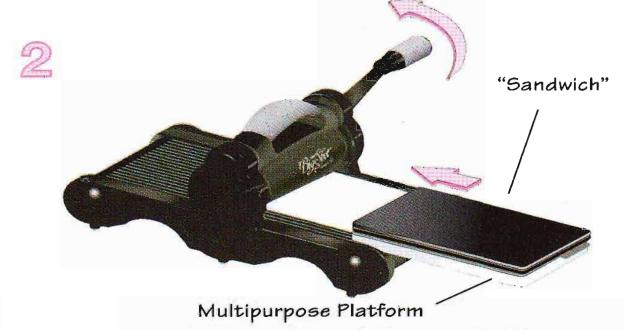
Place the sandwich on top of the Multipurpose Platform and slide both together into the opening of the Big Shot. Note the rotation of the handle and continue to rotate it in the same direction until the sandwich and Multipurpose Platform have passed through the opening and rollers. Remove the Platform from Big Shot, and your embossed design is ready to use!
