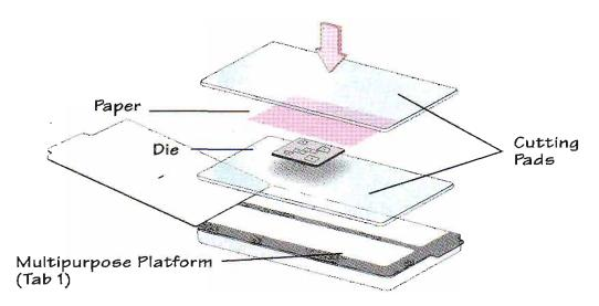
1. Place Sizzlits Die onto a Cutting Pad with foam side up. Place paper over the die. Place another Cutting Pad over the paper to create a "sandwich." For Clearlits Die, place die over photo or material so that the area to be cut shows through the die. Then place photo or material and die between Cutting Pads to make sandwich.
