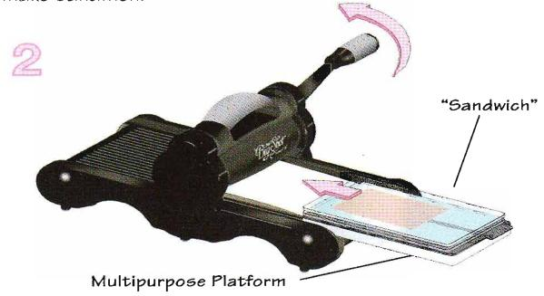
2. Place sandwich on Multipurpose Platform and slide Platform into opening of Big Shot. Note the rotation of the handle and continue to rotate it in the same direction until the Platform has passed through the opening and the rollers. Remove Platform from Big Shot. Your die-cut shape is ready to use!
